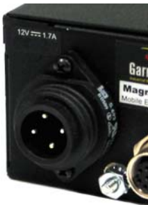
Fig 3.4a Single DC power input
